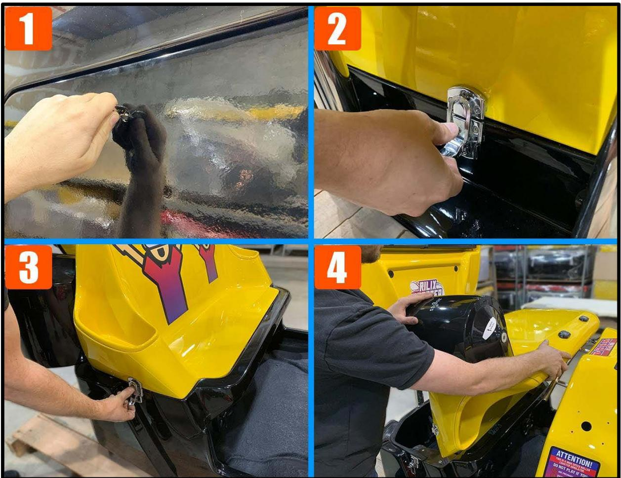
**STEP 7 – INSERTING THE CABLE THROUGH THE INTERNAL BACK DISPLAY PIPE**
