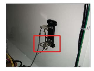
Tilt Alarm: Using Nipper (or similar tools), please cut off the tie around Tilt Alarm
