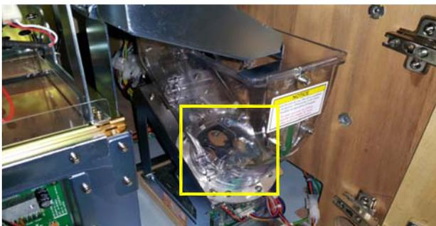
\* CAUSE - ELEVATOR RAIL COIN JAM
