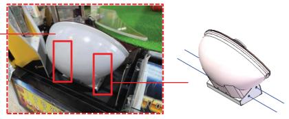
1 Separated into 2 parts on the left and right sides [4 places] - Reuse the removed bolts
