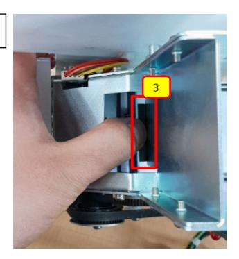
Lock the bolt section 2 pressing upper side of black acrylic between the gaps of No.3 while the card is located.
