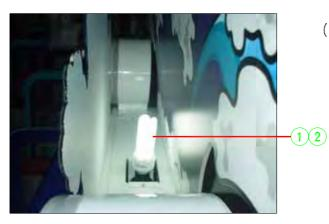
(1) You may change 1 3 WAVE-LAMP after disassemble 2 ACRYL around the lamp.
