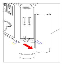
(1) Disassemble 1 "LOWER CORNER ACRYL BRACKET" from front cabinet. (2ea x M6bolt) and change fluorescent light.
