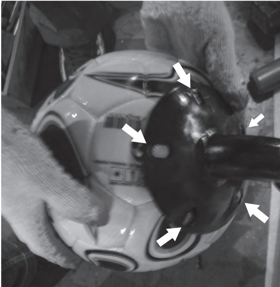
1. Remove the 8mm bolts (total 5) from the ball connector by using 13mm wrench.
