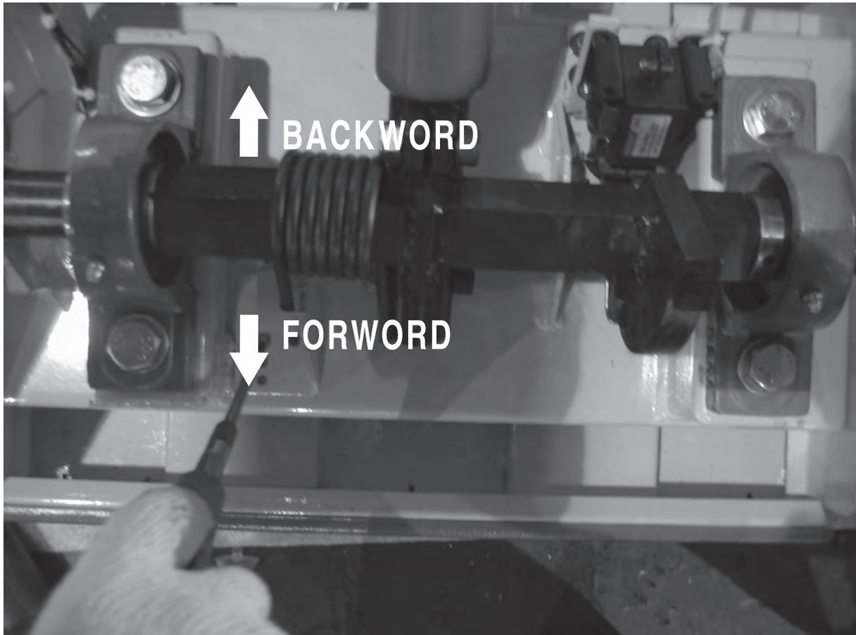
1. If the ball tension is too loose, move the tension control one level **BACKWORD** to make the tension **TIGHT**.
