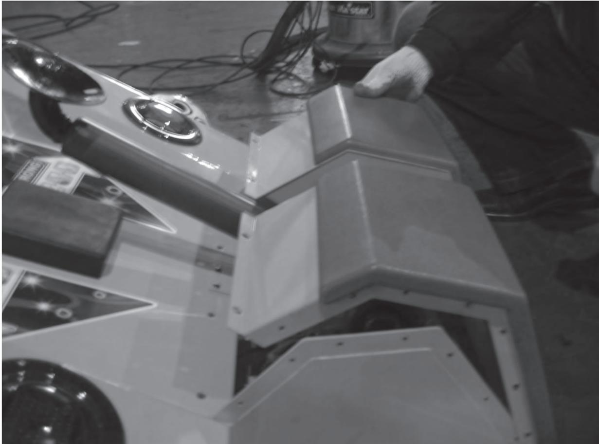
1. Place the bottom of the cover first then fit the upper part of the cover.
