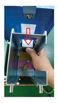
Lock the bolt of section 2 pressing the upper side of black acrylic.
